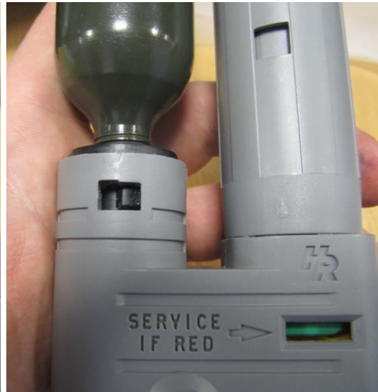
Fig 1.1 – Bayonet Adapter Incorrectly fitted. Cylinder only partially turned. Clip not flush and secured in Firing head mechanism
