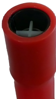
Faulty valve (white cross low in oral tube) simple test try and suck air from the tube
